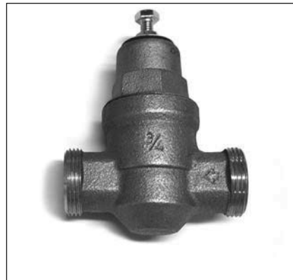
Figure 19 - A Pressure Reducing Valve is required if your home's water pressure is above 80 psi.
